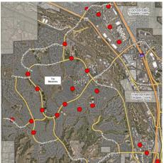
A pre-application request was received seeking information on application and submittal requirements to install 55 small cell wireless nodes throughout the Town of Castle Rock right of way. The small cells would provide wireless network coverage and capacity in areas where macro coverage would not be feasible. The proposed project sites are located throughout all 6 districts.
