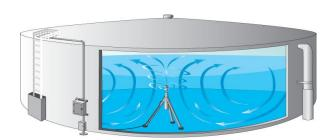
The PAX Water Mixer creates a powerful vortex flow pattern to thoroughly mix the entire tank volume.
