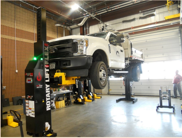
Using our new mobile column lifts to service a 1-ton truck.
