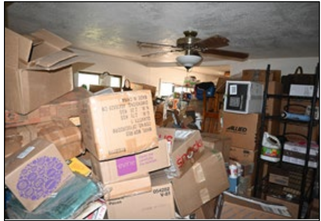
Storage in one portion of a residential home, from floor to ceiling, creating extensive fuel loads and lack of firefighter access to the home.
