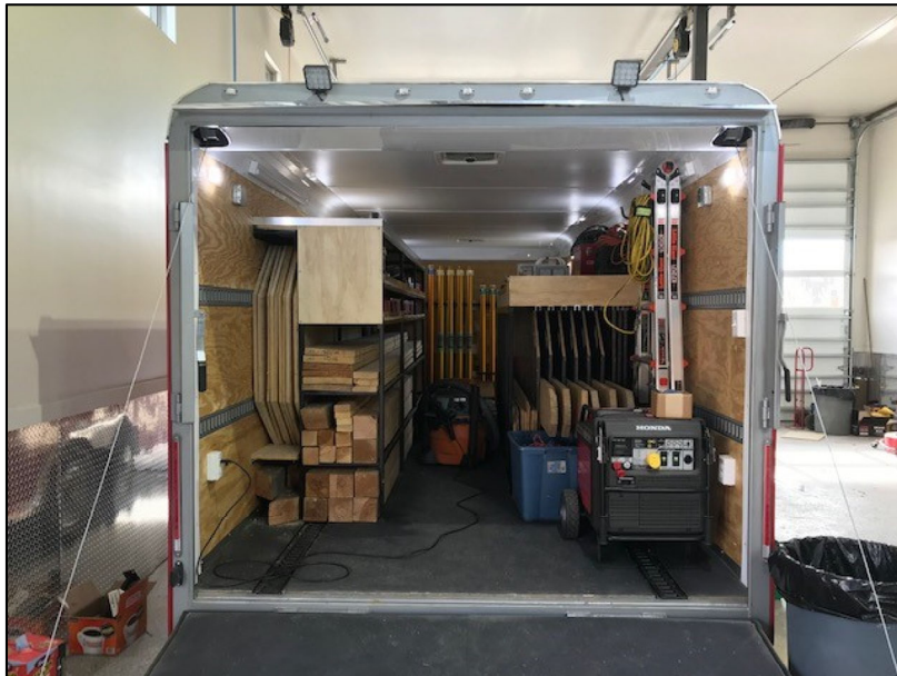
Equipment in the collapse trailer to shore up structures or trenches
