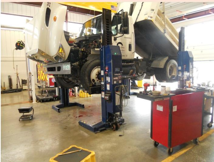
*Fleet technicians using mobile lifts to work on*
