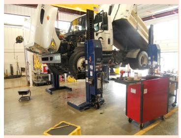
Fleet technicians using mobile lifts to work on
