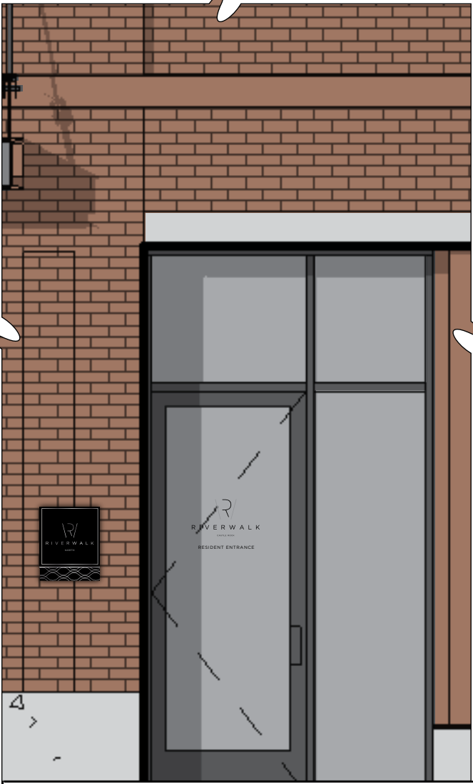
3 North Building Residential Entrance - Partial East Elevation - Scale: 3/8" = 1'
