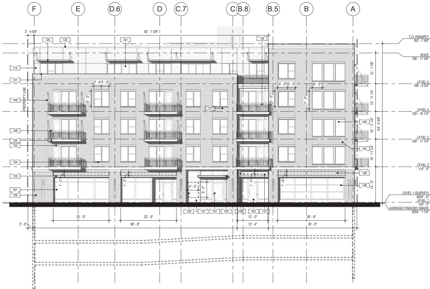
1 BUILDING ELEVATION - EAST 3/32" = 1'-0"
