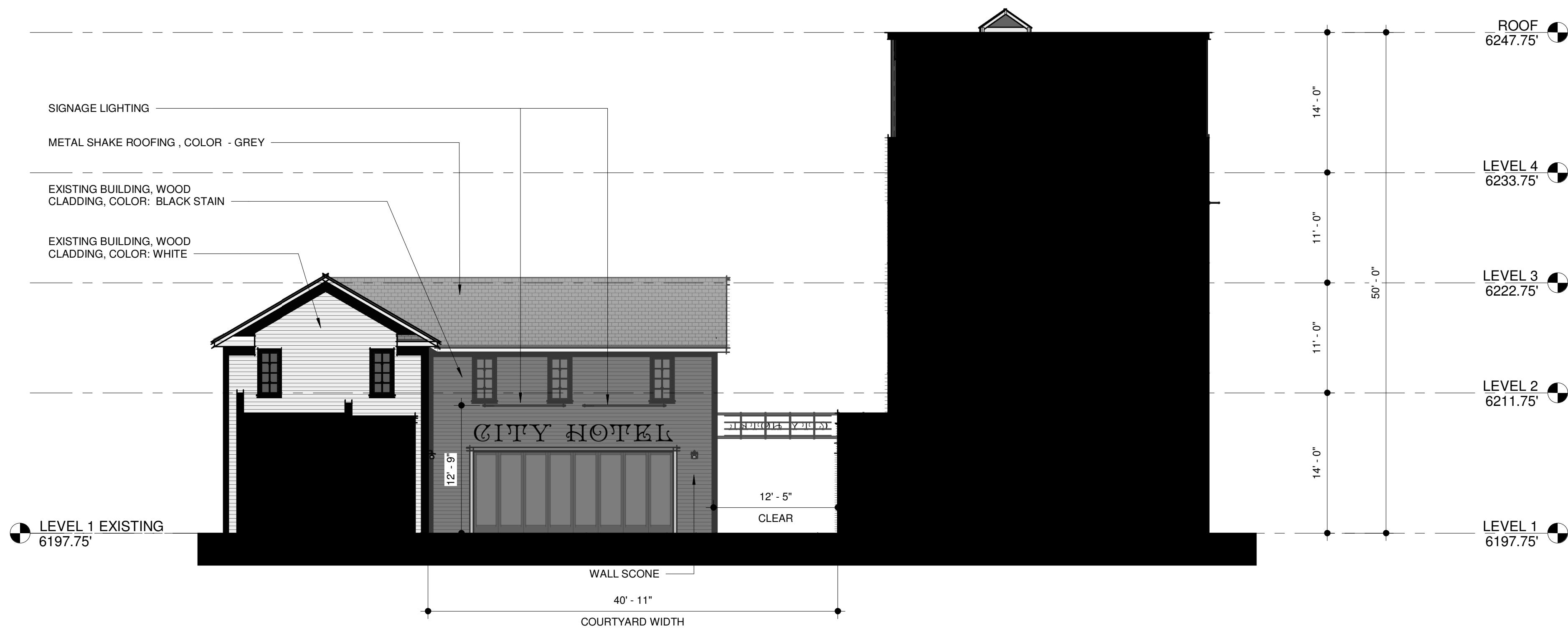
① ELEVATION EAST COURTYARD - SDP 1/8" = 1'-0"
