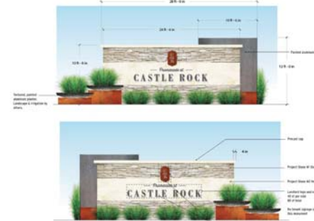
MS18 SIGN FRONT AND REAR ELEVATIONS SCALE: NOT TO SCALE
