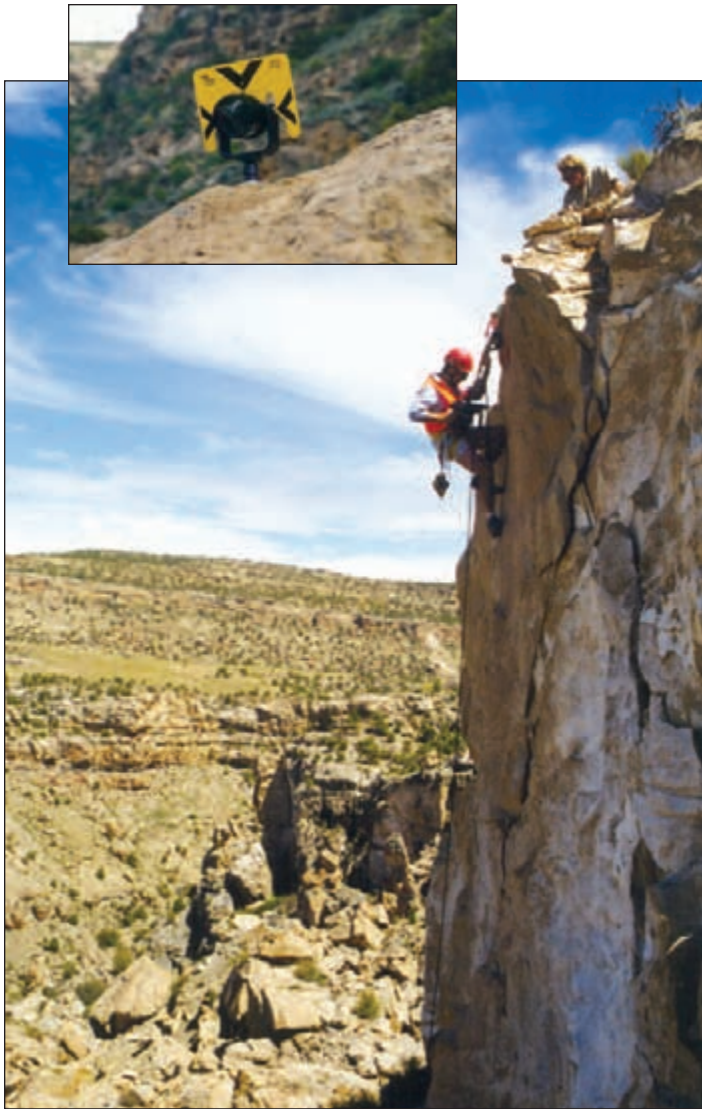
Figure 9: Installation of target prism anchored to a cliff to measure rock movement. Prism is screwed into a wedge anchor bolt that is installed into a drill hole. (Photos by Jon White.)
