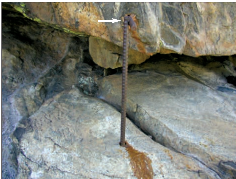
Figure 7: Close up view of tell-tale gauge. Two steel rebar segments (shown with arrow) have been cemented into small drill holes above and below a large crack in the rock. Any movement could be measured by the offset of the two bars that were touching when cemented. This rock has not moved since the gauge was installed in 2003. (Photo by Ty Ortiz, CDOT.)
