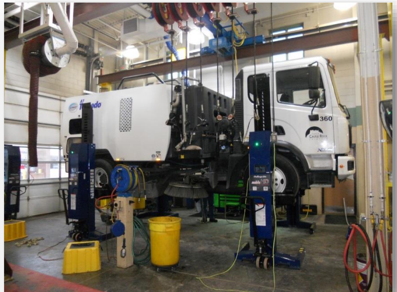
Fleet's new portable lift system being used to work on street sweeper.
