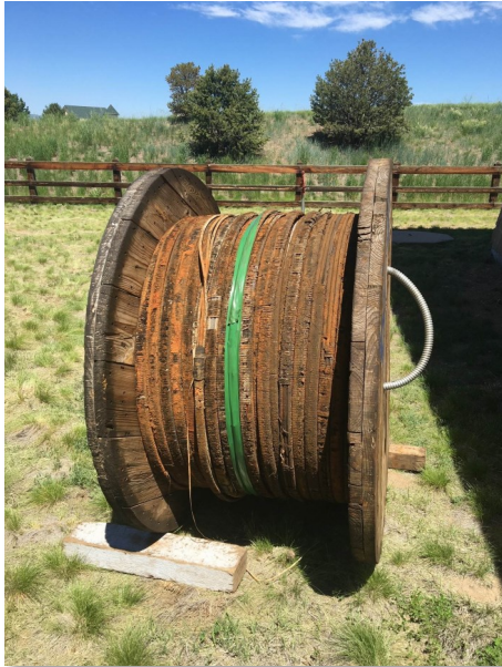
Old cable from Well CR-86 that needed to be replaced
