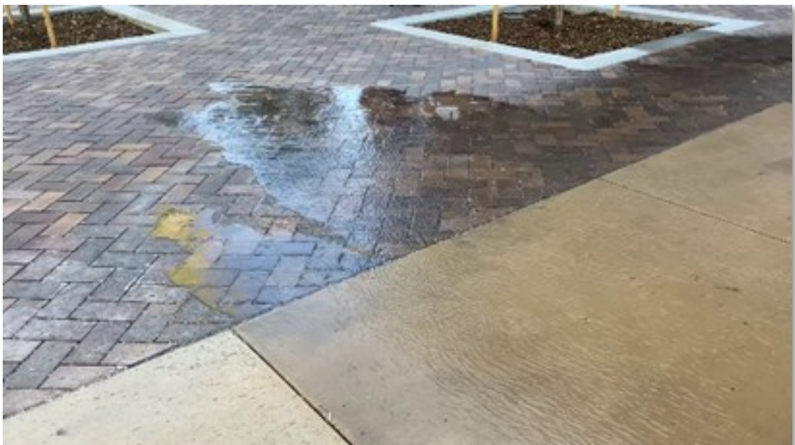
Porous Paver Infiltration over Silva Cells during Demonstration
