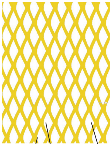
Expanded sheet metal will allow light to pass through areas of the petals so that the flowers can be lit from inside with LED strips to create a colorful glow at night.
