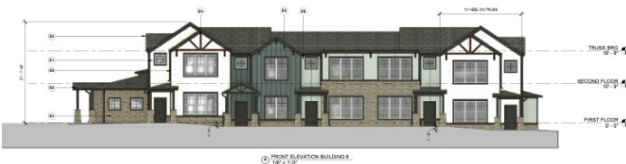
FRONT ELEVATION BUILDING E 1/8" = 1'-0"
