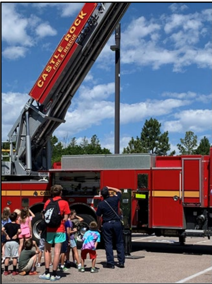
Showing how high the ladder (Quint) truck will reach. It is 105'.
