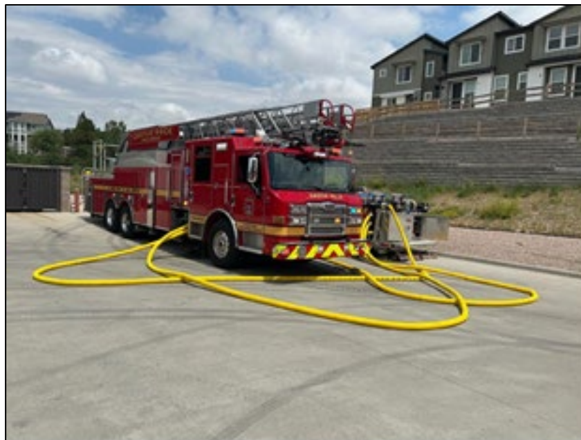
Quint 151 pump testing
