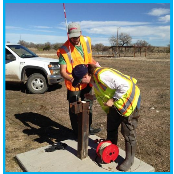
Staff Checking Monitoring Well Levels at Box Elder Well Field
