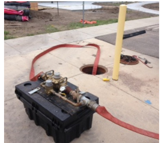
Six-inch meter bench test being conducted at the Justice Center inside the vault
