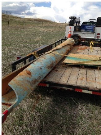
A repair was made to a broken 16" raw water line which feeds water from the North Central Well Field to the water treatment plant. A total of 26 feet of pipe was replaced.
