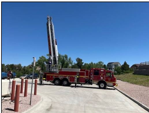
Quint 155 UL Aerial test and inspection
