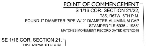
T8S, R67W, 6TH P.M. FOUND BENT #6 REBAR W/ 2-1/2" DIAMETER ALUMINUM CAP STAMPED "LS 6935"
