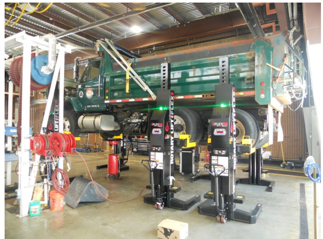
Tandem axle dump truck on new mobile column lifts
