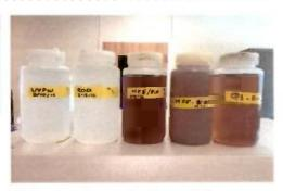
Water samples collected from a full advanced treatment train (MF/RO/UV-AOP, right to left)
