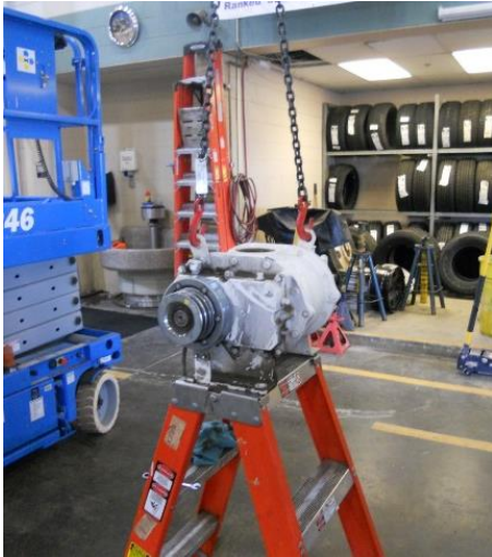
Fleet Techs using overhead crane to remove pump from vacuum unit.
