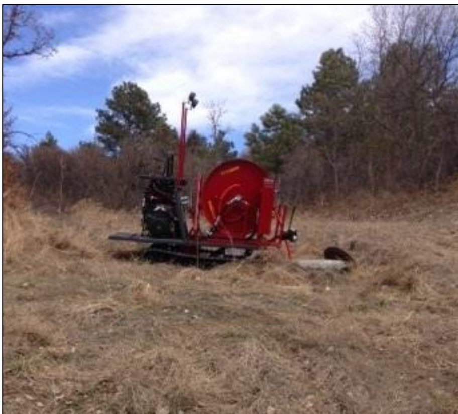
New easement machine to reach out of the way manholes and sewer mains.
