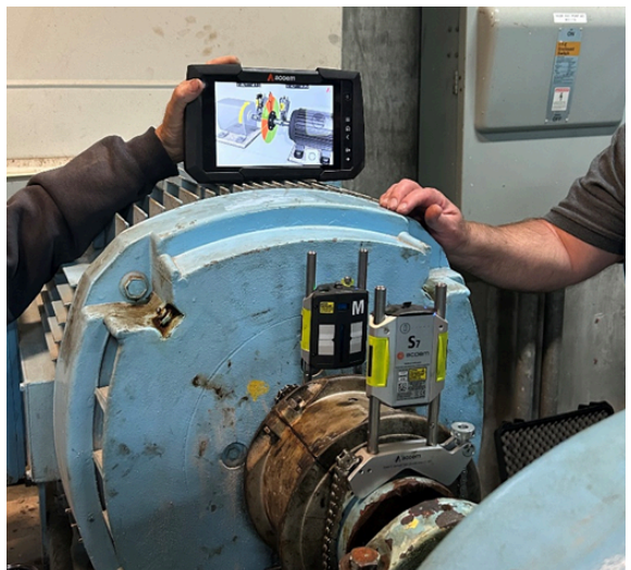
Training for Ops on a new laser alignment tool, which is designed to align shaft motors.
