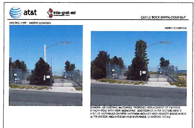
Existing monopole on left, proposed monopine on right
